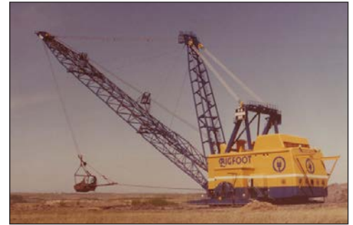
This Bucyrus-Erie 1570-W, along with a Marion 8200, were the two draglines that handled most of the overburden at the Paintearth Mine until closure in 2021.
