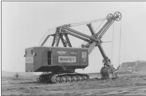
This is the Bucyrus-Erie 190-B shovel that began life in south Wales for G. Wimpey and followed Keith to Canada to work for Luscar Ltd. at the Coal Valley Mine in Alberta.
