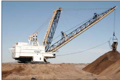
This Bucyrus-Erie 1300-W originally worked for ALCOA in Arkansas with 325-foot boom and 30-yard bucket. In 1994 it was moved to Luscar Ltd.'s Sheerness Mine with shortened boom to accommodate a 46-yard bucket.
